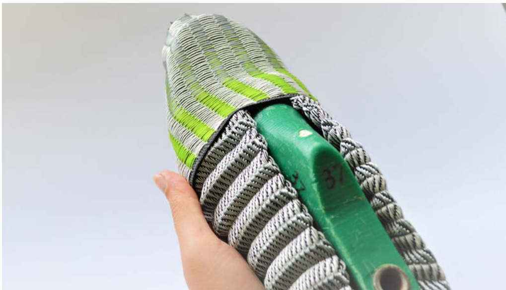
Fig. 15: Examples of weaving technique that creates 3D shapes by incorporating folding lines. © Suzanne Oude Hengel & Milou Voorwinden
