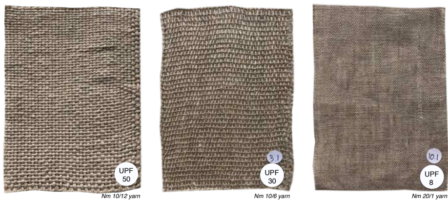
Fig. 14: Examples of woven textile samples with different yarn thickness or openness in the weave © Buro Belén
