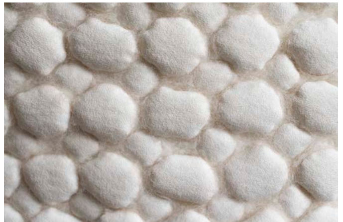
Fig. 12: Examples of 3D shaping textile technologies based on laser cutting, laminating and heat fusing © UNSEAM
